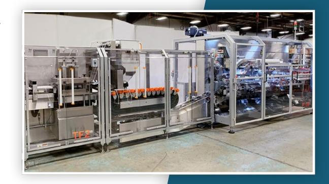
for trays) can easily be switched to the preferred method through a simple changeover of less than five minutes. Its walking beam with dual-sided opposing vacuum ensures square cases all the way through the closing station without the need for flight lugs.
