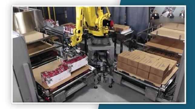
Rejects are ignored by these trained robots and fall harmlessly into a reject bin at the end of the wide pick-and-place infeed belt. Not only does this save QC after flow-wrapping, it also saves the film that would be used to pack out-of-spec or damaged product.
