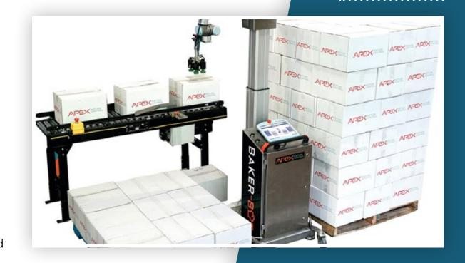
to heavy robot palletizers. The mainframe does not have to be attached to the floor and the RI20 unit can easily be moved using a forklift. The palletizing unit can be relocated in just a few hours, 50% more quickly than alternative solutions the company says, and can be used in multiple lines during the day.
