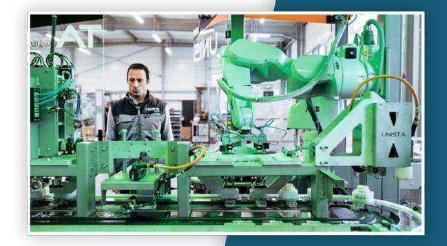
control the dynamic AM8100 servomotors, which are connected via One Cable Technology (OCT). This reduces the cabling costs by 50% and gives the machine a very tidy appearance. A CP3918 Control Panel displays Unista's own user interface.
