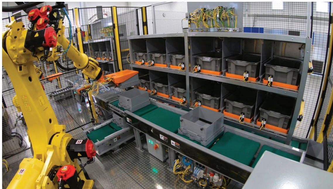
Robot in RFSS placing item in tray.
